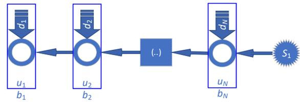
Fig. 2. Serial connection of  $n$  nodes:  $u_1, u_2, \dots, u_N$  – ordering signals and  $d_1, d_2, \dots, d_N$  – imposed demands. Resources are provided by external source  $S_1$ . The arrows indicate the flow of information.
