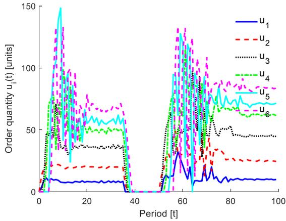
Fig. 11. Order quantity generated at nodes 1–6, under improper records with increased stock level.
