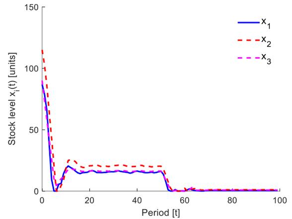
Fig. 22. The stock level at nodes 1–3, under improper records with increased stock level, Network A.
