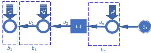
Fig. 3. BE calculation in a serial connection of  $N$  nodes with internally ( $u_1, u_2, \dots, u_N$ ) and externally ( $d_1, d_2, \dots, d_N$ ) imposed demand.
