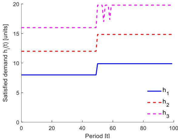
Fig. 20. Satisfied demand at nodes 1–3, under improper records with increased stock level, Network A.
