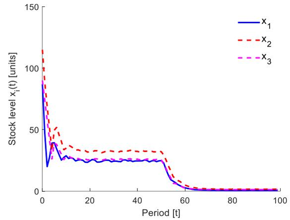
Fig. 19. Stock level at nodes 1–3, under improper records with reduced stock level, Network A.
