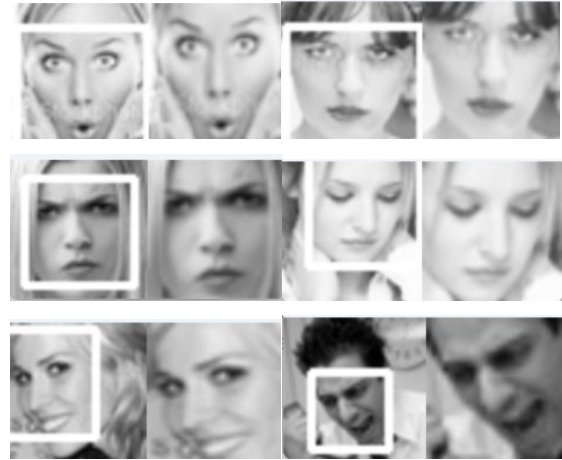
Fig. 1. Examples of facial images detected and adjusted to 48x48 pixel size, with unimportant details removed for training.
