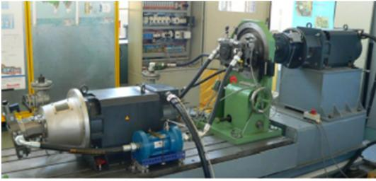
Fig. 2. HST test rig at the Chair of Mechatronics, University of Rostock.
